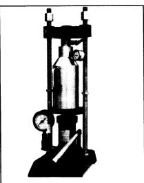
Figure 1. Hydrostatic pressure chamber and press used to treat fertilized eggs to produce triploid fish.
