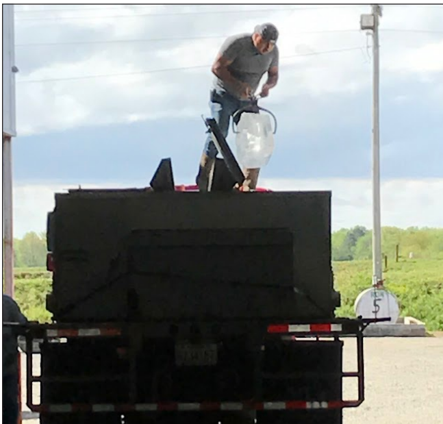
Figure 2. Adding ice to the hauling tank to reduce water temperatures.
