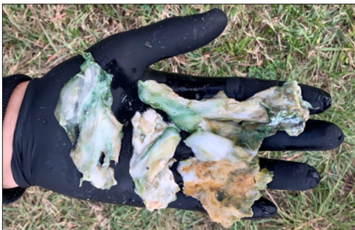
Figure 2. If left untreated, water containing hydrogen sulfide (H 2 S) may create a “slime” that can compromise aquatic animal health and create system maintenance issues.
