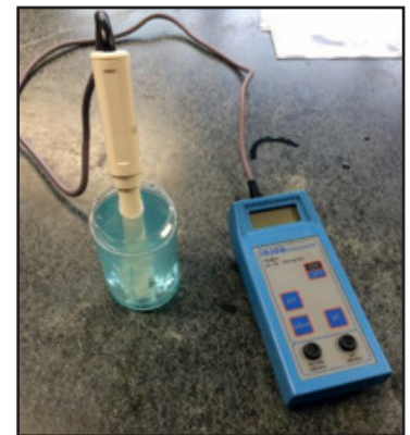
Figure 12. An electrical conductivity (EC) meter is used to monitor and check fertilizer concentrations.
