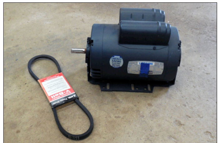
Figure 13. Spare motor and fan belt.
