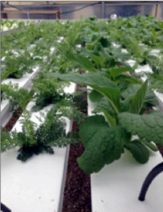
**Figure 4.** Commercially manufactured NFT production channels.
