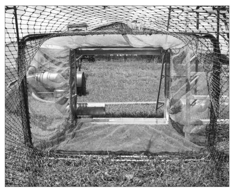
Figure 3. Inside view of the eduction chamber with attached live car. The 8-inch water jet (bottom left) moves the fish across the eduction chamber and into the 14-inch, urethane, flex-duct assembly (bottom right). The 14-inch, urethane, flex-duct assembly connects to the in-pond grader.
