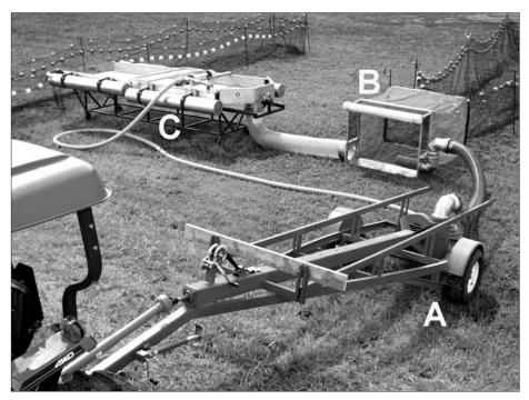
*Figure 2. Components of the in-pond fish grading system: A) a trailer with an integrated, 8-inch, re-lift style water pump; B) a fish eduction chamber; and C) a floating, adjustable, horizontal bar grader.*
