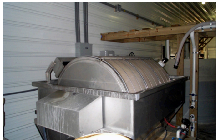
Figure 5: A microscreen with spray nozzles mounted in the rear of the unit.
