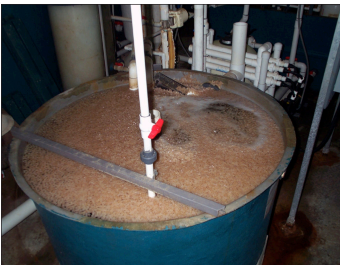
Figure 7: A Moving Bed Reactor supported by a bank of UV lights on a marine fingerling system.
